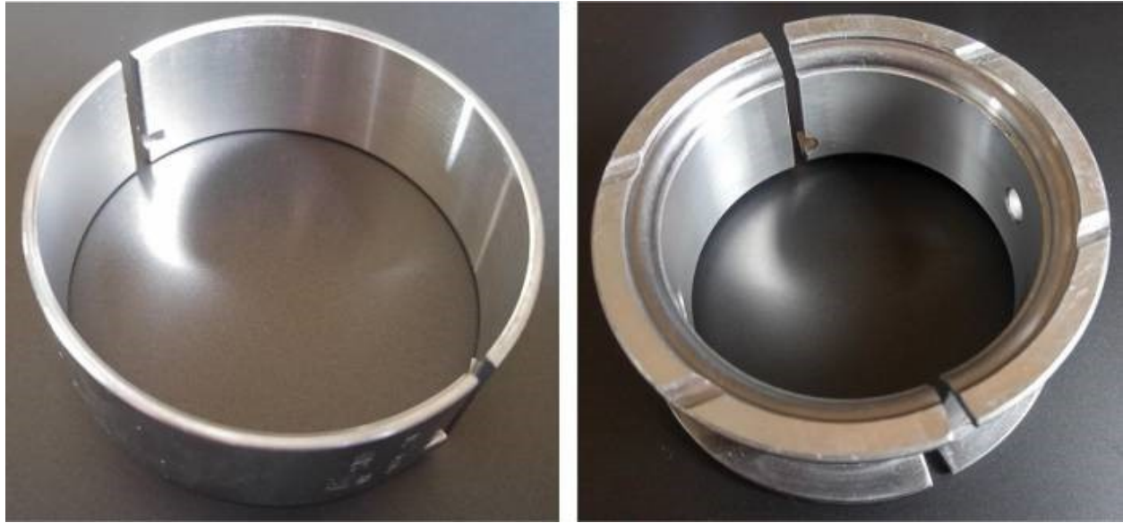
Fig.3 Bimetallic Engine Bearings with Aluminum Lining
