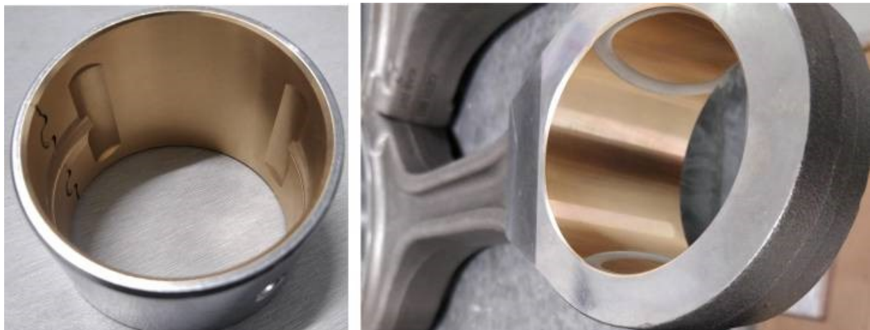
Fig.7 Bimetallic Bushings with Bronze Lining
